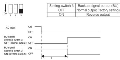
Backup signal output (BU) delay time setting (setting switches 1, 2)
